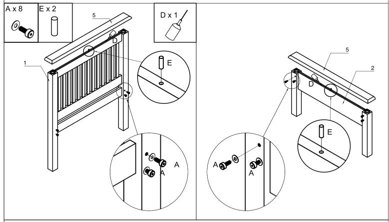
**Step 2:** Slide the metal hooks on the side rails over the screws in the headboard (1) and footboard (2). Now, tighten each of the eight screws at the headboard (1) and footboard (2). The bed frame should be very solid when the screws are tightened
