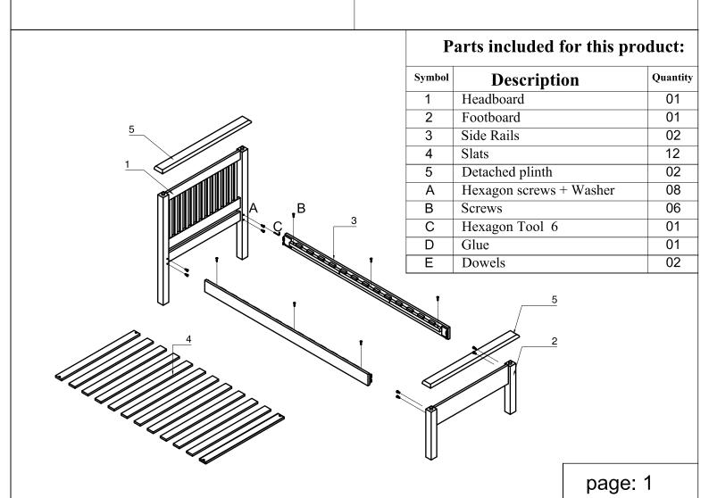
**Step 1:** Using the Hexagon Tool (C), insert the hexagon screws (A) into the headboard (1) and the footboard (2). Note: Turn each screw approximately 4 or 5 rotations only for now. They will be tightened later.
